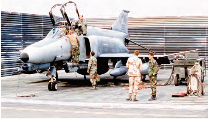
The crew of 561st TFS F-4G 69-0265 is about to strap in for the redeployment flight to George. The first 12 aircraft departed Shaikh Isa on March 22. The Weasel's configuration included an AN/ALQ-184 ECM and luggage pods. (USAF, Sgt Jeff Wright)
