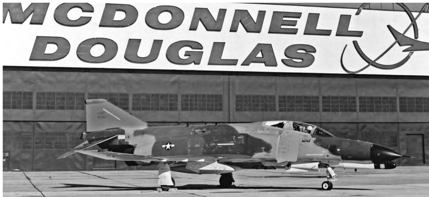
Block 43 F-4E 97254 of the 414th Fighter Weapons Squadron (Nellis) was selected as prototype for the R&D phase of the F-4E AWW program. Earlier it had served as kit-proof F-4E for the Leading Edge Slats modification. It is seen here at McAir in St. Louis in December 1975, prior to departing for Edwards for phase II of the DT&E. (McAir)
