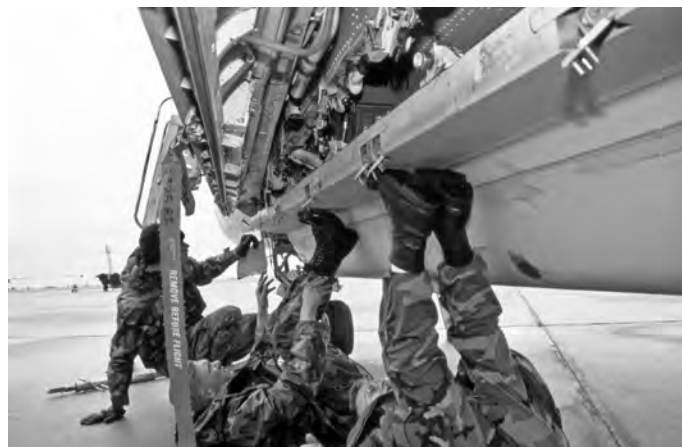
These 366th TFW maintainers were not exercising to improve their PT grades, but were trying to close the doors of the canoe-shaped radome manually. It was mounted under the fuselage, occupying the old bomb bay space and housed the antennas for the high-powered jamming transmitters. (Guy Aceto)
