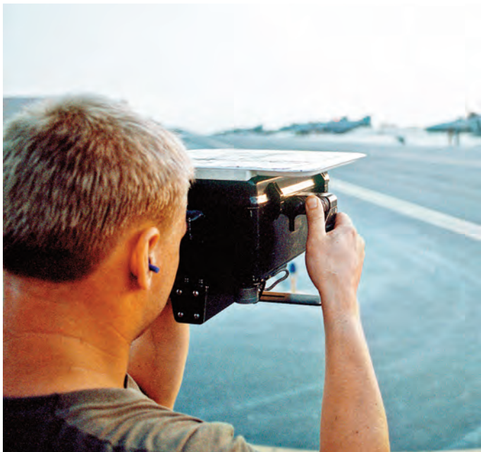
Sgt. Todd Nelson of the 52nd TFW is checking the Mode 4 on an F-4G on the parking ramp area. Mode 4 is a military discrete variant of ATC's Identification Friend or Foe (IFF) used throughout the world. Mode 4 is an encrypted IFF, changed daily, and thus the reason for being checked before takeoff, especially when used in combat operations. (USAF, MSGt Bill Thompson)
